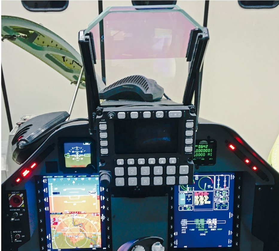
Head-Up Display, PDU-159-01 in the front cockpit of the L-39NG (SkyFox)
